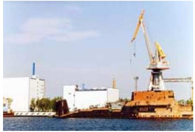
*Section of special quay with portal crane of 80 tons lifting capacity*
