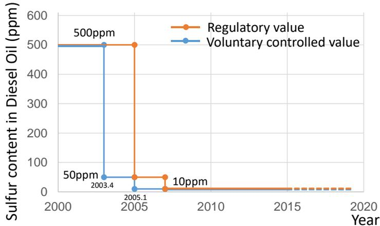
Figure 6. Changes in Sulfur Content of Diesel Fuel
