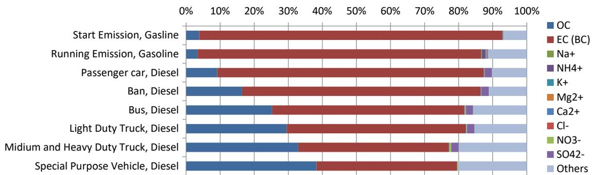
Figure 4. Component analysis of PM<sub>2.5</sub> emitted from vehicles
