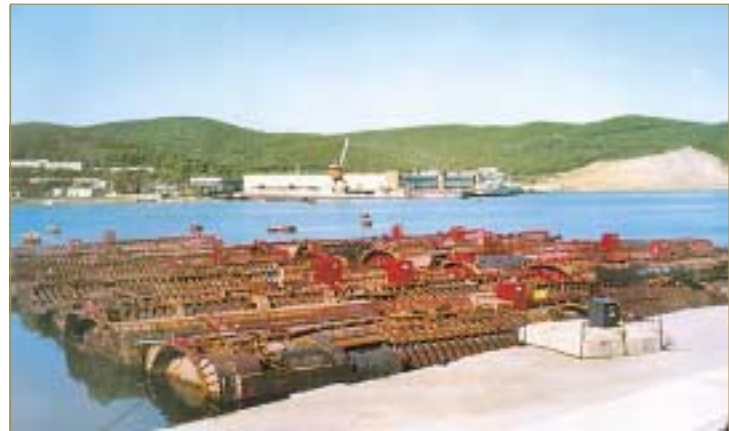
Storage of three-compartment reactor blocks afloat in Razboyinik Bay
