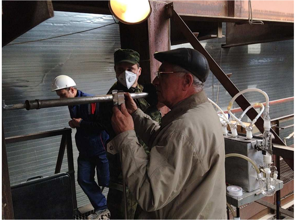
The probe is introduced into the duct by the measuring team
