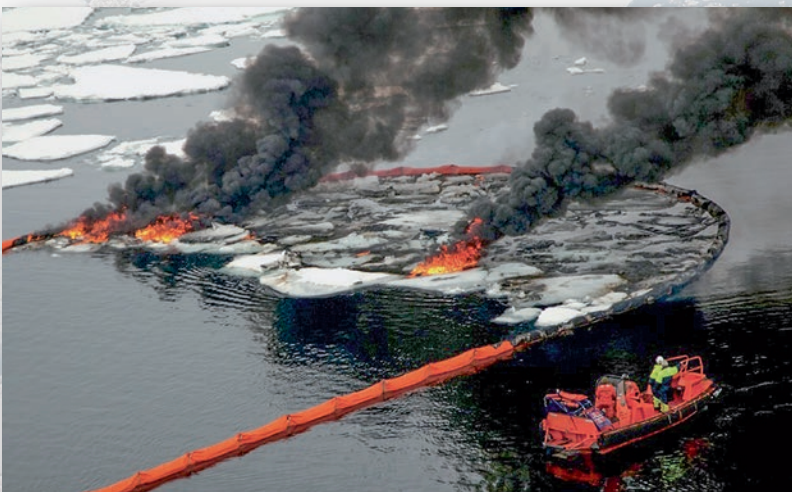
Burning crude oil spilled into a field of small ice cakes collected in a fire-resistant boom – Norway 2009.
