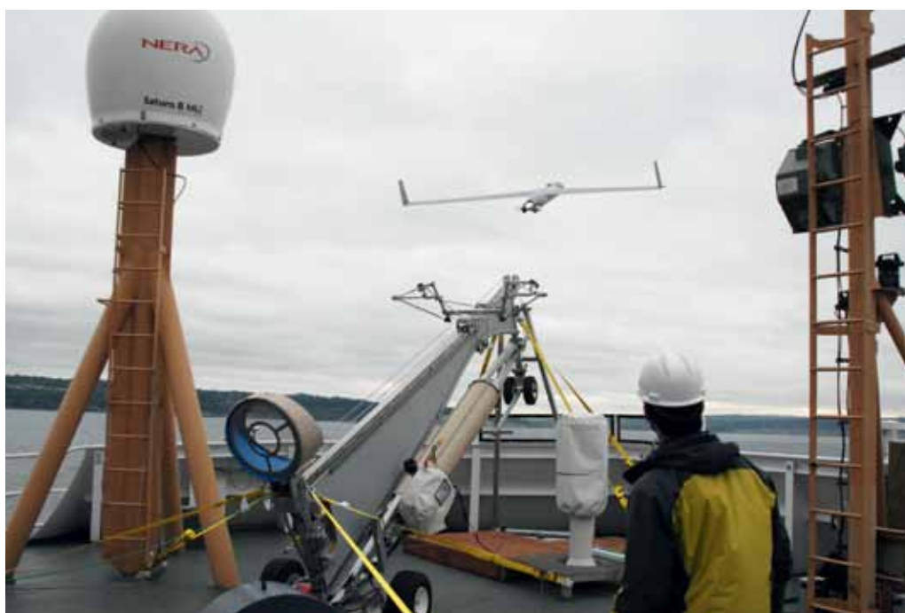
Figure 6.1. UAS platforms are versatile and portable. The upper photo shows Scan Eagle being deployed from a launching system onboard a research vessel at sea, while the lower photo shows Cryowing and Mantra ready for takeoff on land in Ny-Ålesund, Svalbard, 2011. Photos courtesy of the U.S. National Oceanic and Atmospheric Administration (NOAA) (upper) and Kjelle-Sture Johansen, Norut (lower).
